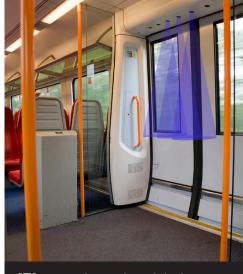
STS system shown above is in the **Command to Open** function: when passengers place their hands anywhere within the detection zone, STS signals to open the doors (providing that the doors have been enabled).
